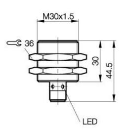
Inductive Sensors BES 516-327-E5-Y-S 4 M30x1.5 x 44.5 normally-open Sn=10mm shielded
